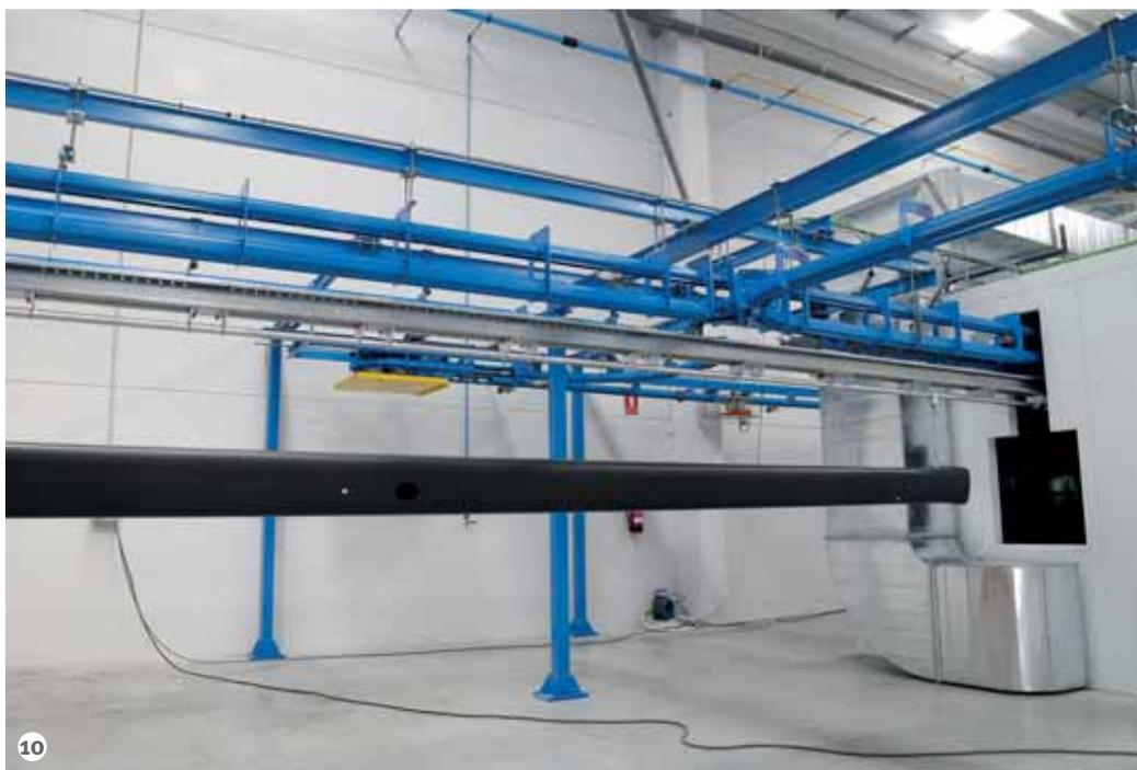
**Figure 10: Each load bar can carry up to two workpieces at a time.**
