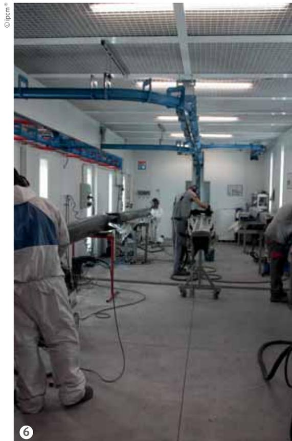
Figure 6: The booth with the sanding stations.
