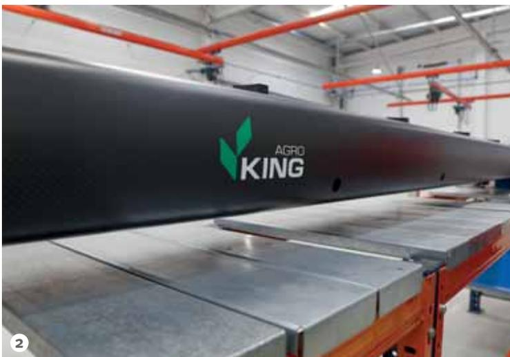
Figure 2: A carbon fibre spray boom.
