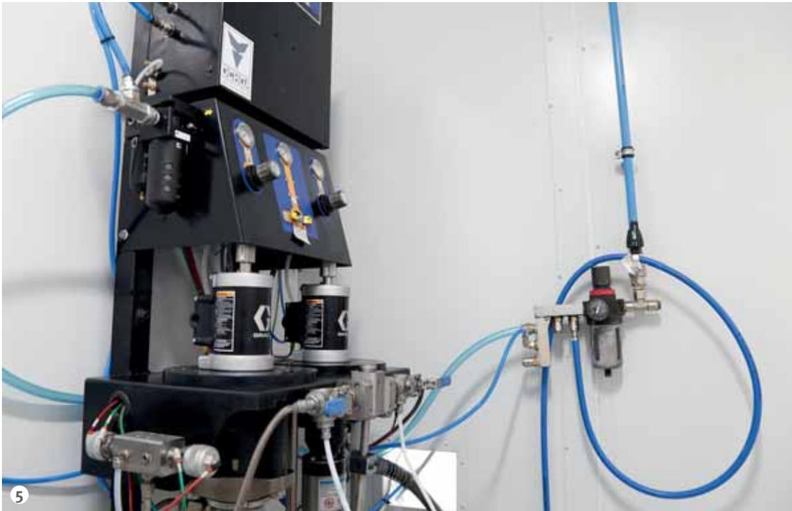
Figure 5: The mixer for two-component coatings (Graco).
